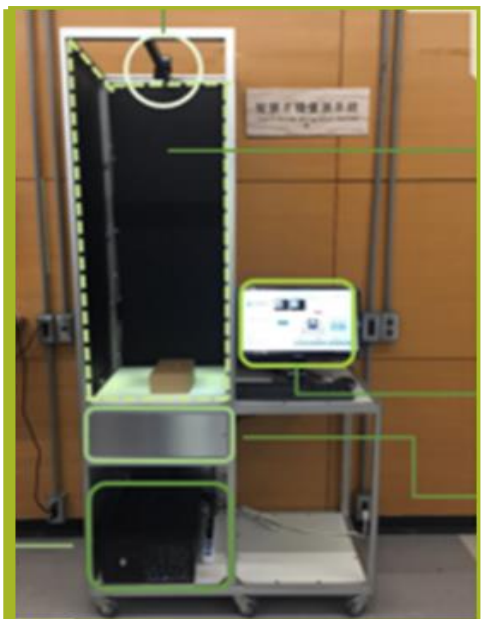
智慧才積 量測系統 Smart Volume Measurement System
